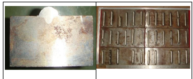
Figure 1. shows the welding profile and work pieces of weld bead
