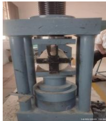
Figure 2. Split Tensile test setup
