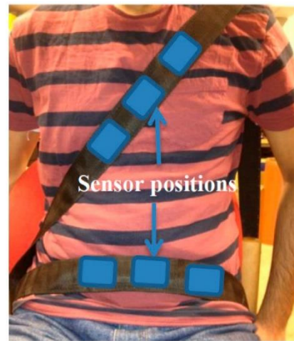
Fig. 2. Sensors integrated in seat belt
