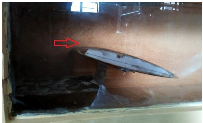
Figure 2. Smoke moves at 25° angle of attack
