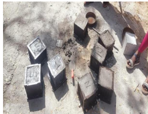
Figure 1. Casting of Specimens
