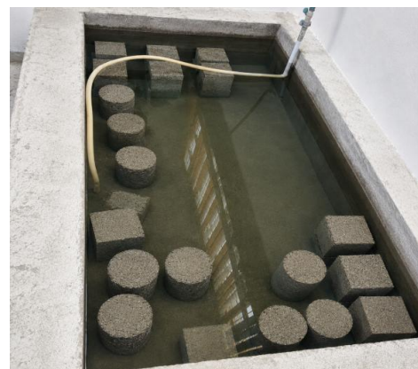
Figure 2. Curing of Specimens
